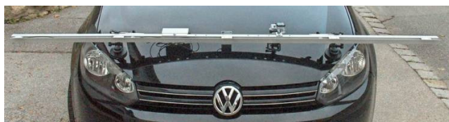
Figure 1: LimeCam Sensor-Rack, attached to vehicle.
